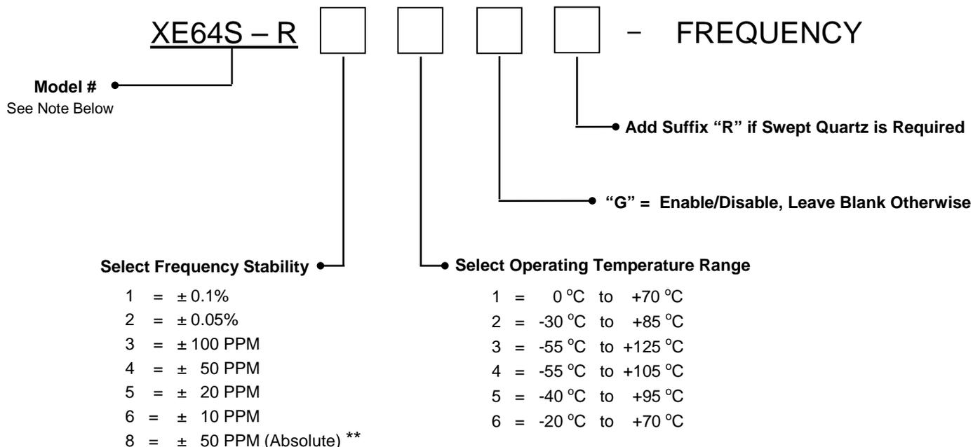
\*\* Option 8 provides ± 50 PPM frequency-temperature stability referenced to the specified nominal frequency including load & supply voltage variations of ± 10%.
