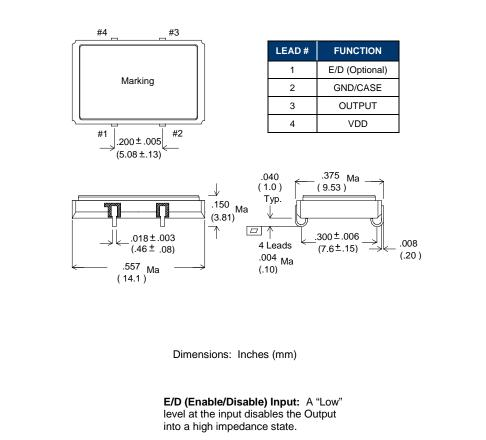
E/D Input has internal pull-up, it can be left floating or connected to Vdd.
