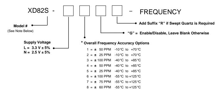
\* Overall Frequency Accuracy includes effects of Operating Temperature, Supply Voltage, Load variations and 5 year aging
