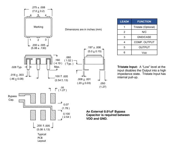
Figure 1 - Package Configuration & Pin Connections
