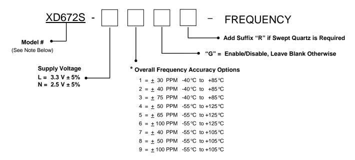
\* Overall Frequency Accuracy includes effects of Operating Temperature, <u>+</u> 5% Supply Voltage & <u>+</u>10% Load variations.
