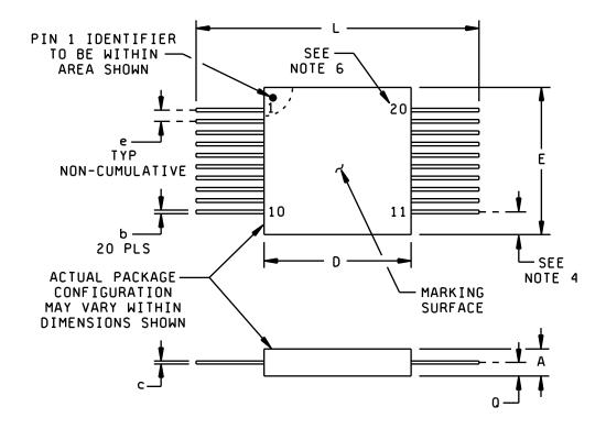
FIGURE 1. <u>Dimensions and configuration</u>.
