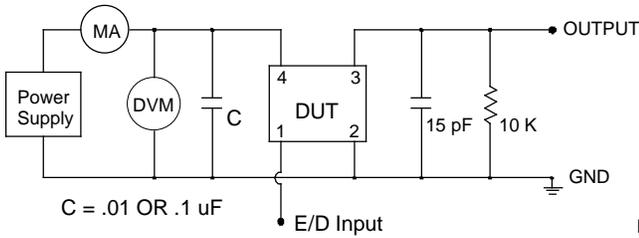
**E/D ( Enable/Disable ) Input** has an internal pull-up resistor. It can be left floating or connected to Vdd.
