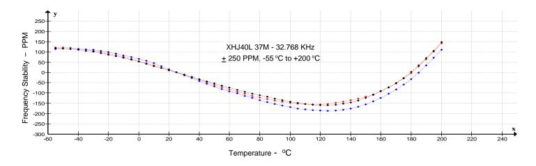
32.768 KHz, Real Time Clock Oscillator
