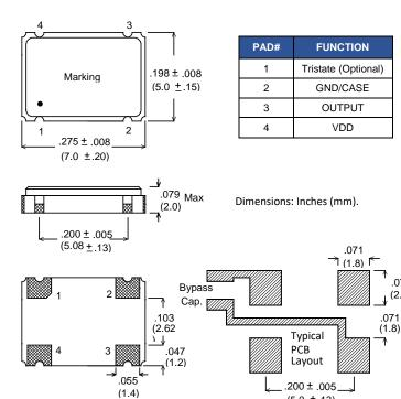
Tristate Input: A "Low" level at the input disables the Output into a high impedance state.
