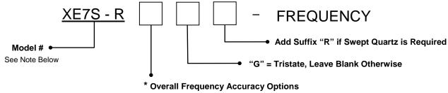
1 =  $\pm$  50 PPM -10 °C to +70 °C 2 =  $\pm$  25 PPM -10 °C to +70 °C 3 =  $\pm$  100 PPM -40 °C to +85 °C 4 =  $\pm$  50 PPM -40 °C to +85 °C 5 =  $\pm$  25 PPM -40 °C to +85 °C 6 =  $\pm$  100 PPM -55 °C to +125 °C 7 =  $\pm$  75 PPM -55 °C to +125 °C 8 =  $\pm$  60 PPM -55 °C to +125 °C
