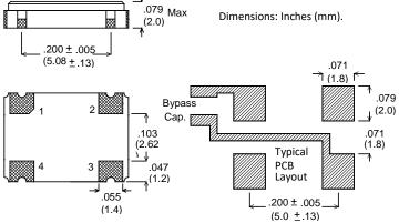
Figure 1 - Package Configuration & Pin Connections
