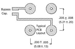
An External 0.01 µF Bypass Capacitor is required between VDD and GND.
