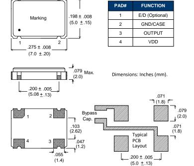
**Tristate Input:** A "Low" level at the input disables the Output into a high impedance state.
