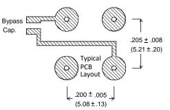
An External 0.01 µF Bypass Capacitor is required between VDD and GND.
