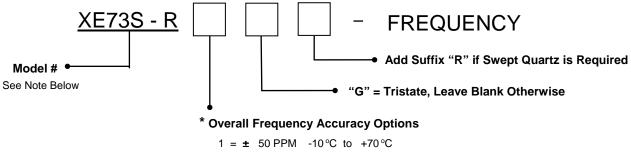
1 =  $\pm$  50 PPM -10 °C to +70 °C 2 =  $\pm$  25 PPM -10 °C to +70 °C 3 =  $\pm$  100 PPM -40 °C to +85 °C 4 =  $\pm$  50 PPM -40 °C to +85 °C 5 =  $\pm$  25 PPM -40 °C to +85 °C 6 =  $\pm$  100 PPM -55 °C to +125 °C 7 =  $\pm$  75 PPM -55 °C to +125 °C 8 =  $\pm$  60 PPM -55 °C to +125 °C
