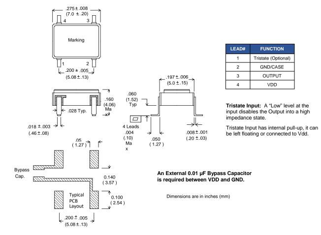
Figure 1 - Package Configuration & Pin Connections
