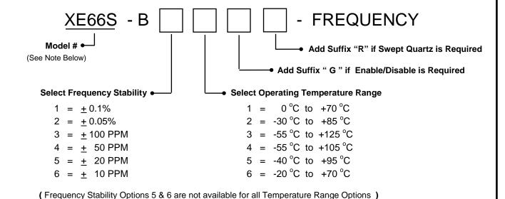
P/N Example: XE66S - B43 - 24.000 MHz = 24.000 MHz, Class "S" Oscillator, ± 50 PPM Frequency Stability over an operating temperature range of -55 °C to +125 °C,
