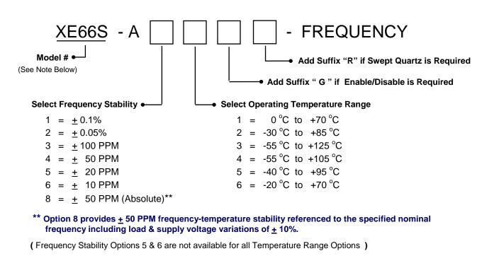
P/N Example: XE66S - A43 - 24.000 MHz = 24.000 MHz, Class "S" Oscillator, <u>+</u> 50 PPM Frequency Stability over an operating temperature range of -55 °C to +125 °C,
