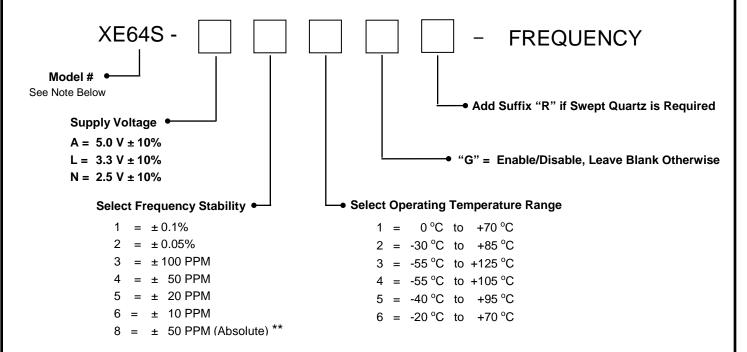
\*\* Option 8 provides ± 50 PPM frequency-temperature stability referenced to the specified nominal frequency including load & supply voltage variations of ± 10%.
