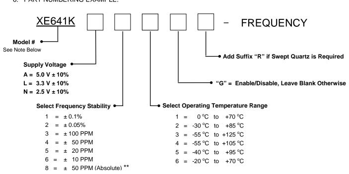
\*\* Option 8 provides ± 50 PPM frequency-temperature stability referenced to the specified nominal frequency including load & supply voltage variations of ± 10%.
