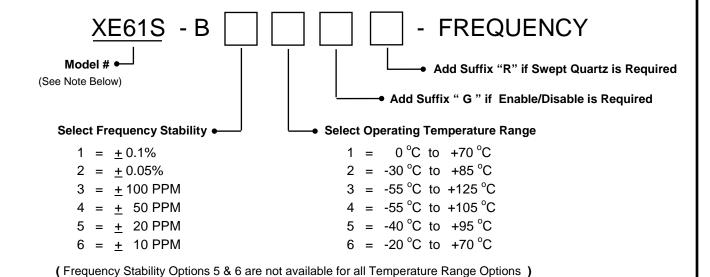
P/N Example: XE61S - B43 - 24.000 MHz = 24.000 MHz, Class "S" Oscillator, ± 50 PPM Frequency Stability over an operating temperature range of -55 °C to +125 °C.
