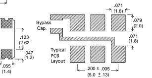
Figure 1 - Package Configuration & Pin Connections
