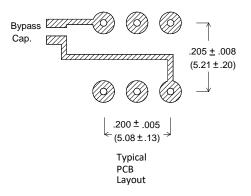
An External 0.01uF Bypass Capacitor is required between VDD and GND.
